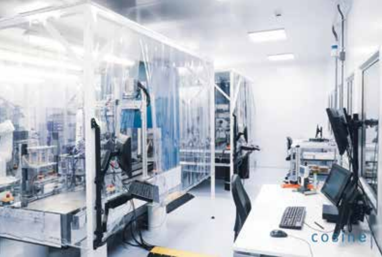
Left: cosine cleanroom where Silicon Pore Optics are stacked and bonded. Right: Silicon Pore Optics module in cosine cleanroom.
