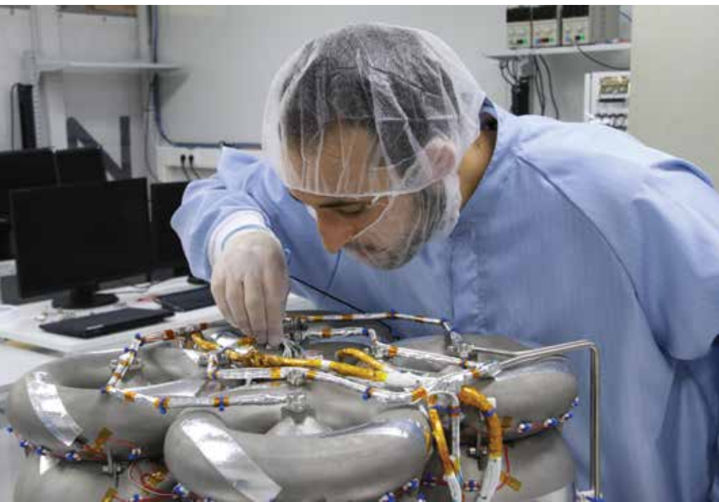
Top: the Dawn team with the Aurora Mk-II spaceplane demonstrator. Left: the SatDrive propulsion module with tanks, components and engine during assembly. [Dawn Aerospace] Bottom left: the 20 N B20 thruster is one of the main products of Dawn Aerospace. [Dawn Aerospace]
