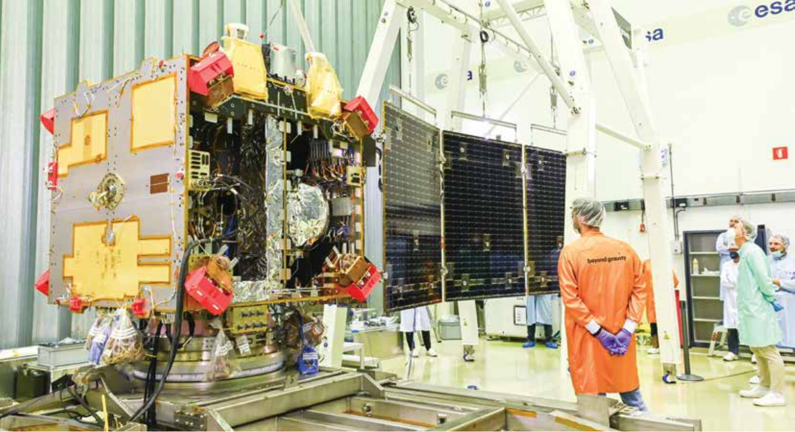
Hera with one of its two solar wings added, during the test campaign at the ESTEC Test Centre. [ESA-SJM Photography]
