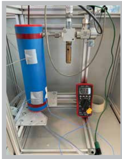
Left: Proba-2 satellite assembly, the four cool gas generators are visible at the centre. [ESA] Right: Prototype of the EVE Oxygen Generator. [HDES]
