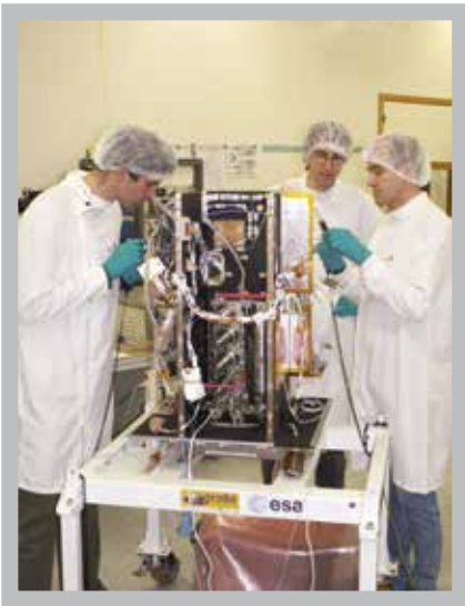
Left: Proba-2 satellite assembly, the four cool gas generators are visible at the centre. [ESA] Right: Prototype of the EVE Oxygen Generator. [HDES]
