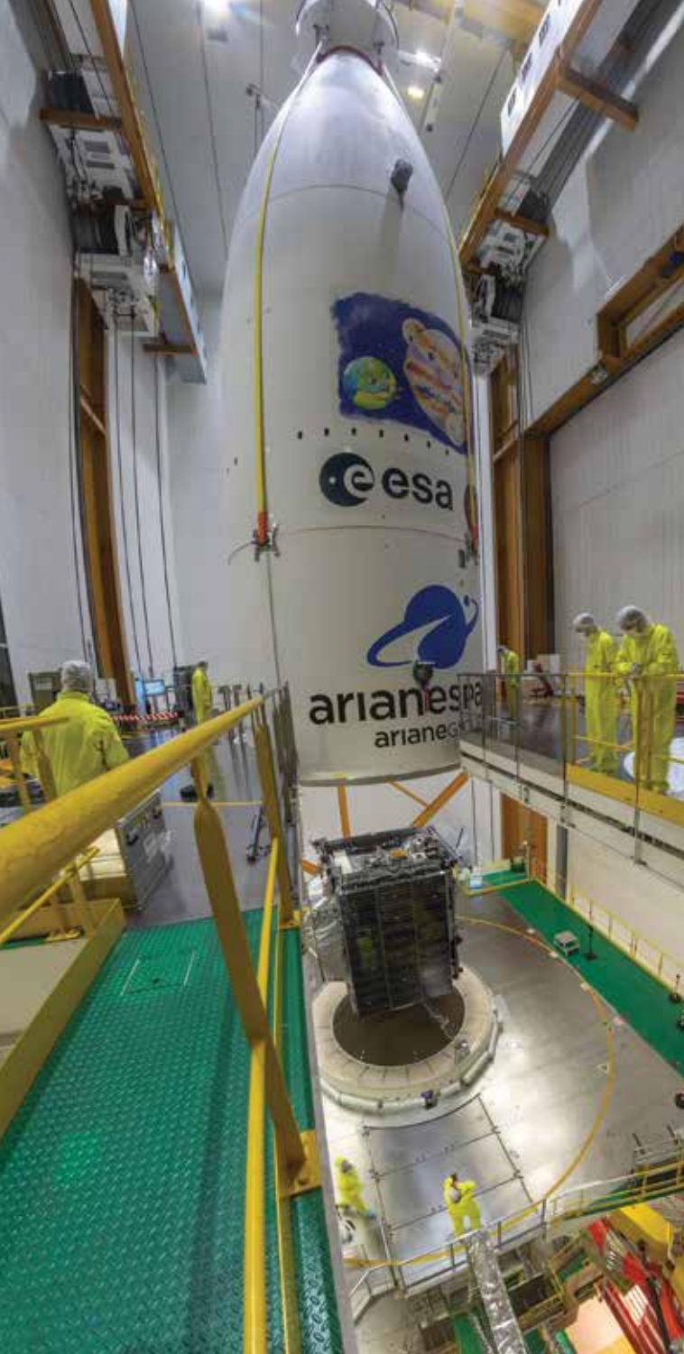
Left: JUICE being encapsulated into the Ariane 5 fairing. [CNES/Arianespace] Right: JUICE is launched. [CNES/Arianespace]
