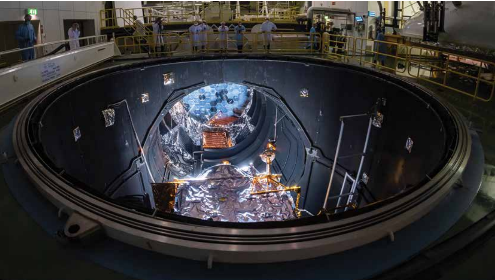
Top left: JUICE shortly after arrival in ESTEC, being readied for testing. [ESA/Airbus Defence and Space] Top right: preparation of JUICE for thermal vacuum testing at ESTEC. [ESA/ADS] Bottom: the spacecraft in the Large Space Simulator in ESTEC, during an illumination test. [ESA]
